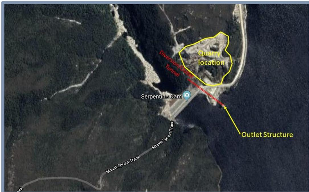
Serpentine Dam has an existing gated outlet for spill from Pedder Impoundment and could be used to dewater that section of the impoundment. Its maximum capacity is 243m<sup>3</sup>/s which is sufficient for current spill operations of the reservoir in conjunction with McPartlan Pass Canal but an assessment would need to be done should Serpentine Dam remain with a lower FSL as this will be the only outlet.
