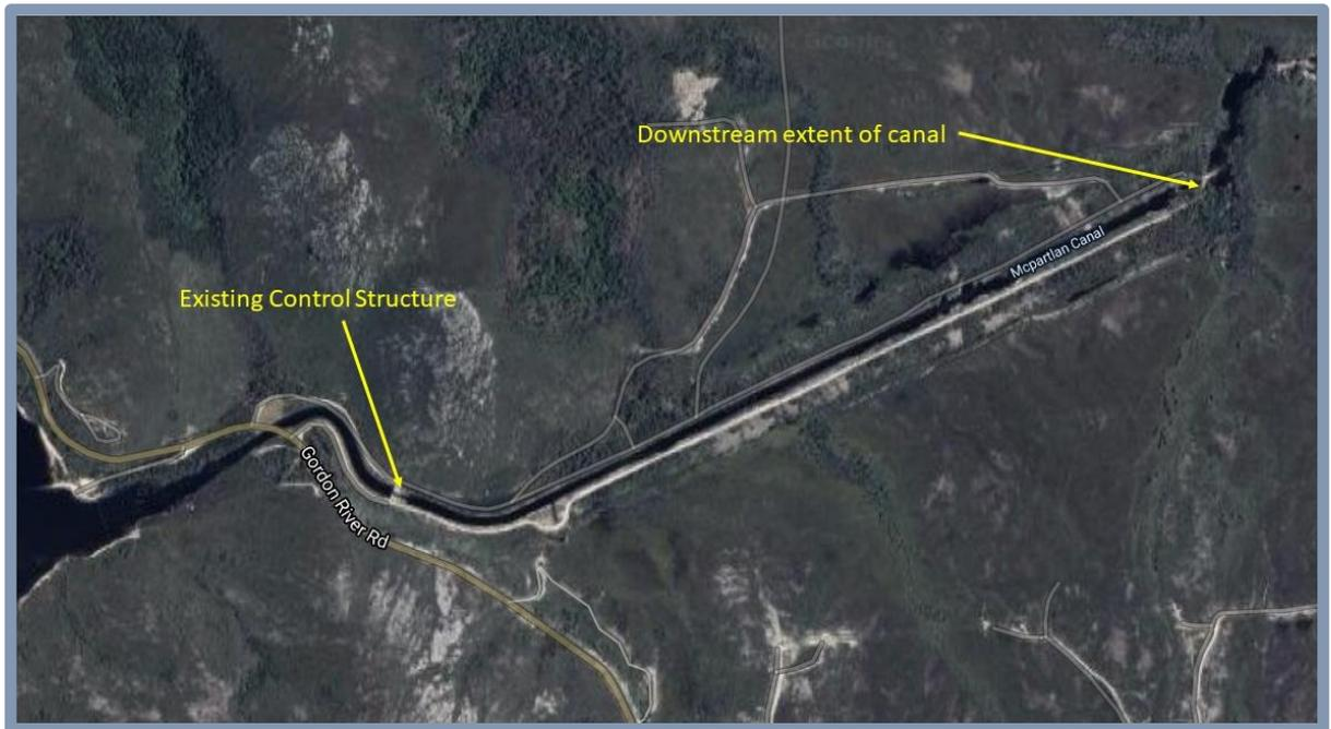
The engineering would need to consider a fish barrier to prevent the spread of red fin, an exotic fish species that is currently controlled by maintaining constant flow levels from the Huon-Serpentine Impoundment to Lake Gordon.
